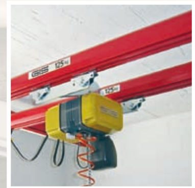
Double bridge suspended crane
