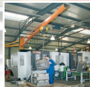
Slewing pillar crane
