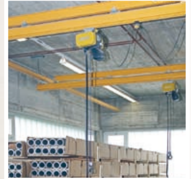
Single bridge suspended crane
